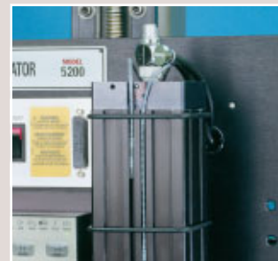
3 Improved tamp assembly allows the unit to be set-up and adjusted quickly and easily.
