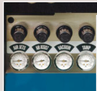
5 Easy-access controls and gauges enable operator to adjust and monitor air supply.
