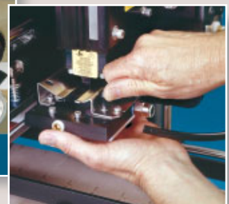
6 Quick-change tamp pad allows for easy replacement to accommodate different label sizes.
